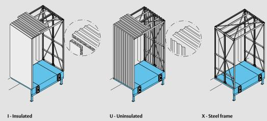
For optimal insulation the I-insulated type is provided with 40 mm insulated cladding.
